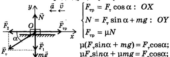
$$\left[ \begin{array}{l} F_{\text{тр}} = F_t \cos \alpha : OX \\ N = F_t \sin \alpha + mg : OY \\ F_{\text{тр}} = \mu N \end{array} \right]$$
